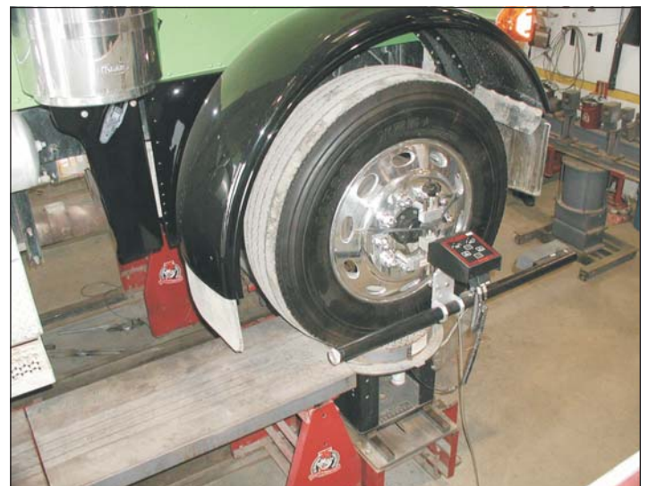
Photo 7: State-of-the-art front and rear axle laser alignments include before and after readings of castor, camber, toe in, ackerman angles, KPI and turn angles.
