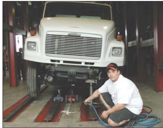
Photos 5 & 6: Frame rack setups showing the process of straightening a severe twist from the front and rear.
