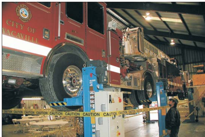
Photo 1: West Coast Frame has the capability of lifting a three-axle tiller for inspection and repairs.
