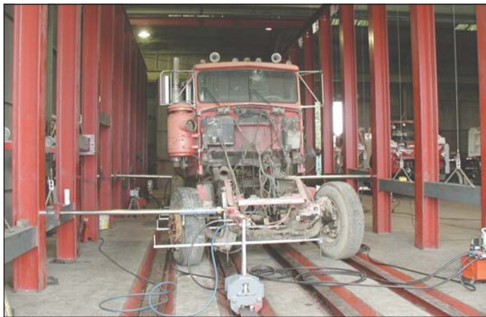
Photo 4: Their frame rack has the capability of having multiple setups and functions at the same time.
