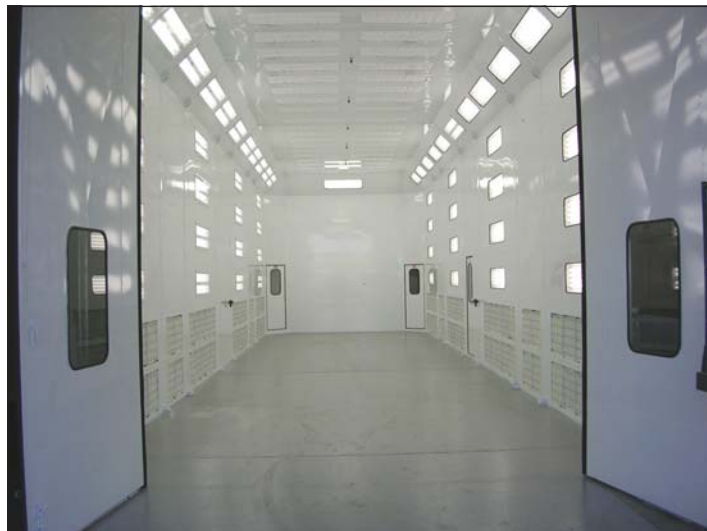
Photo 3: WCF's 60-foot downdraft paint booth for factory clean paint jobs from simple to complex.
