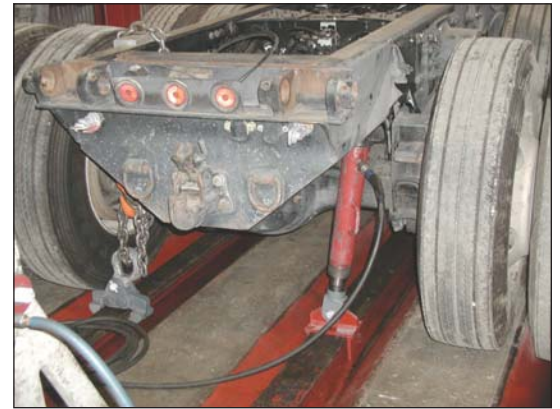
Photos 5 & 6: Frame rack setups showing the process of straightening a severe twist from the front and rear.
